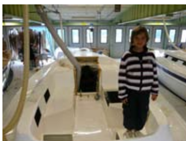
Deck and hull have been screwed and laminated together before interior work
